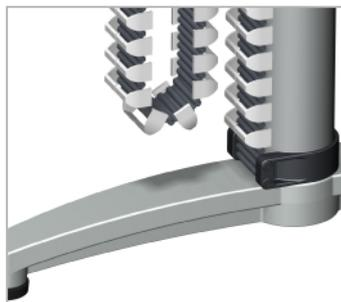
respectively at the top and bottom of the upright tube and align them loosely. Tighten the cable chain and the screws.
