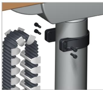
Mount the plastic panel with the cable chain. Mount the cable chain and clamp with 4 screws
