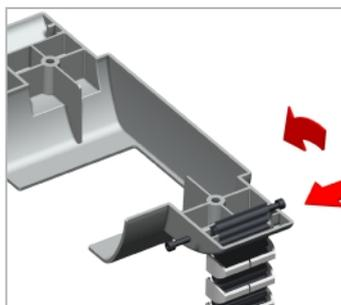
Detach the plastic panel; insert the cable chain through the slot and secure it by mounting the screws.
