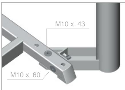
Tighten screws to torque of 35 Nm!
