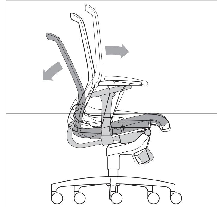
synchronous leaning backwards and forwards from -12° to 0°, or includes activating an opening angle of up to 5° in the seat and an up to 26° tilt in the back. At the same time, the seat and back can be tilted sideways from the horizontal by up to 13°. The counter pressure provides support in any direction and infinite adjustment of the elasticity allows it to adapt to people weighing between 45 to 140 kg.
